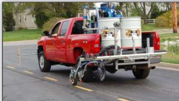
RAE Paint is available in 55-gallon drums and 275-gallon totes for GRACO's truck-mounted RoadPak™ Sprayer and other long-line applications.
