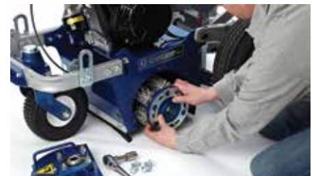
3. Remove drum assembly
